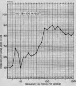
Figure 4. Vibration spectrum at pump.
