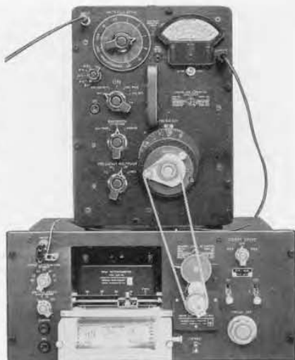
Figure 7. View of the analyzer with dial drive coupled to the Type 1521-A Graphic Level Recorder.
